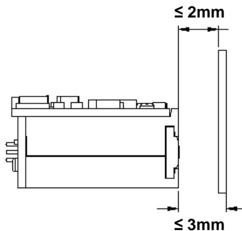
If the window is required to be in a tilted position, the above distance requirements should be met and tilt angle should ensure no reflections back into the lens.
